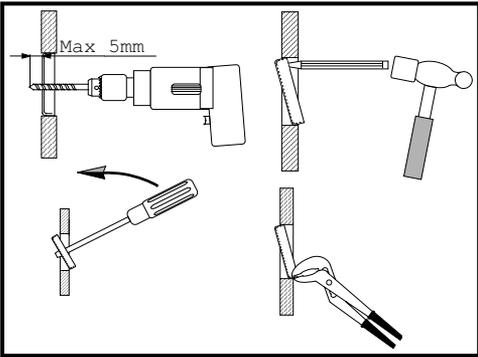
(EN) Drain the coolant. Remove the frost plug which covers the hole as shown in the figure. This can be done by drilling an 8-10 mm hole in the middle of the plug and then prising it out with a drift or similar. Insert the engine heater in the hole and tighten it in place with the attaching parts supplied. Fill up with coolant and vent the cooling system. Run the engine and check that there is no leakage.
